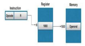
From above example, it is clear that, the instruction(MOV AL, [BX]) specifies a register[BX], and in coding of register, we see that, when we move register [BX], the register contain the address of operand(1000H) rather than address itself.
