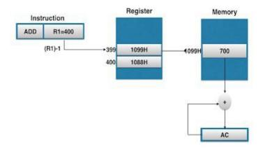
Here, we see that, in the Auto-decrement mode, the register R1 is decremented to 399 prior to execution of the instruction, means the operand is loaded to accumulator, is of address 1099H in memory, instead of 1088H. Thus, in this case effective address is 1099H and contents loaded into accumulator is 700.
