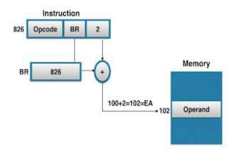
Thus, the difference between Base and Index mode is in the way they are used rather than the way they are computed. An Index Register is assumed to hold an index number that is relative to the address part of the instruction. And a Base Register is assumed to hold a base address and the direct address field of instruction gives a displacement relative to this base address.
